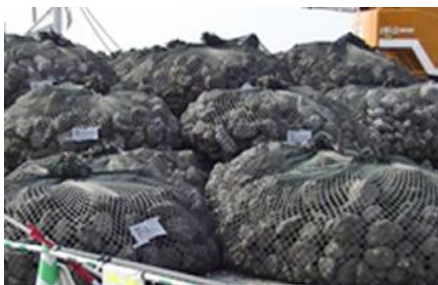
Submerged breakwater construction material using steel slag
