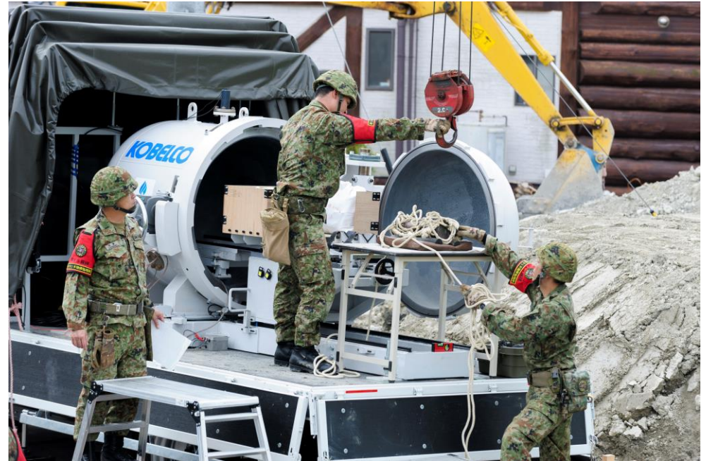
Disposal of UXO using an explosion-resistant container for 5-inch naval gun shells
