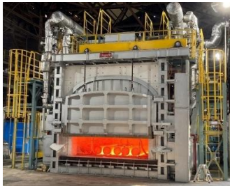
Introduction of a hydrogen-fueled metal heating demonstration furnace with Japan's largest combustion capacity
