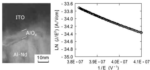
(a) Cross-sectional TEM image at the interface between ITO/Al-Nd (b) I-V characteristics of ITO/Al-Nd contact
