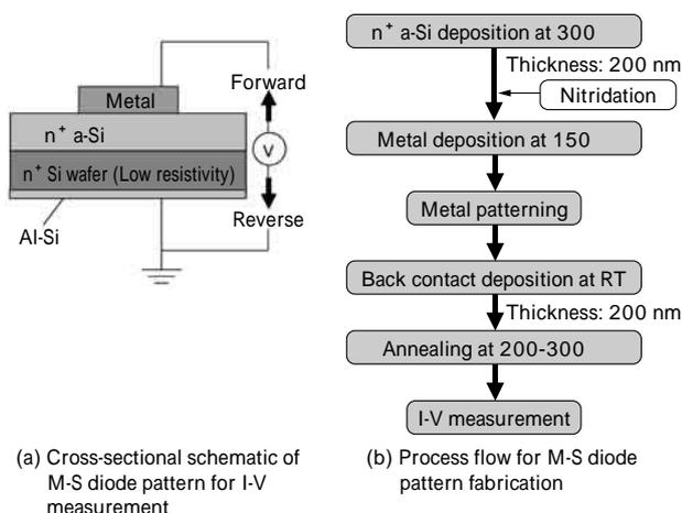
Fig. 5 Evaluation of I-V characteristics using M-S diode device
