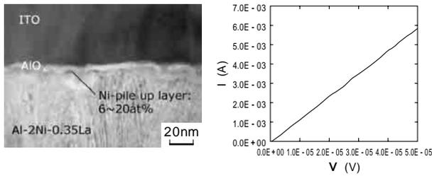
(a) Cross-sectional TEM image at the interface between ITO/Al-2at%Ni-0.35at%La (b) I-V characteristics of ITO/Al-2at%Ni-0.35at%La contact
