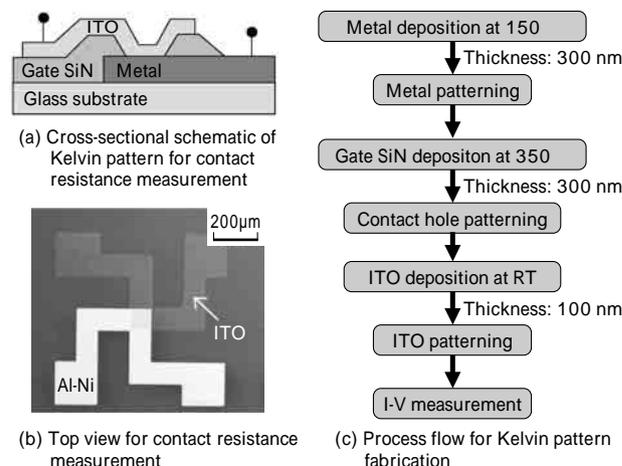
Fig. 4 Evaluation of contact resistance measurement using Kelvin pattern device
