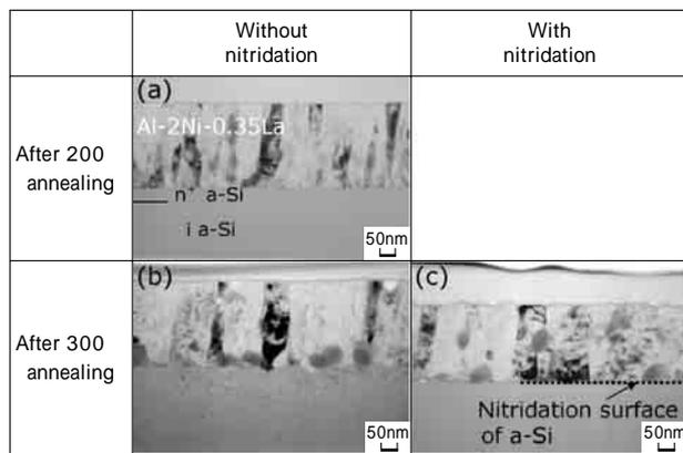
(a) Al-2at%Ni-0.35at%La after 200 annealing (b) Al-2at%Ni-0.35at%La after 300 annealing (c) Al-2at%Ni-0.35at%La after 300 annealing with nitridation of a-Si
