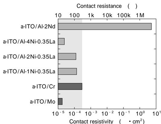
Fig. 7 Comparison of the contact resistance for various metals with ITO
