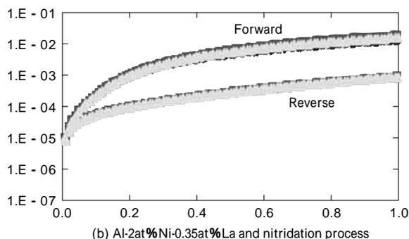
Fig.11 Forward and reverse I-V characteristics of M-S diode
