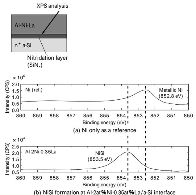
Fig.10 XPS analyses at Al-2at%Ni-0.35at%La/a-Si interface
