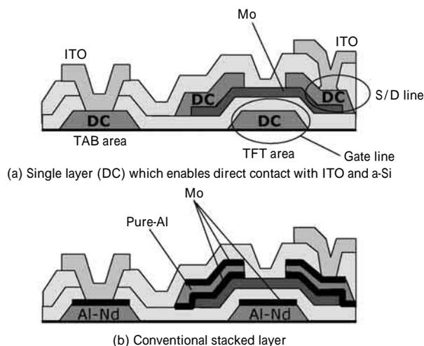
Fig. 1 Schematic configuration of cross-sectional TFT
