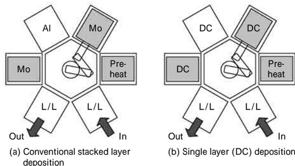
Fig. 2 Cluster-tool sputtering equipment
