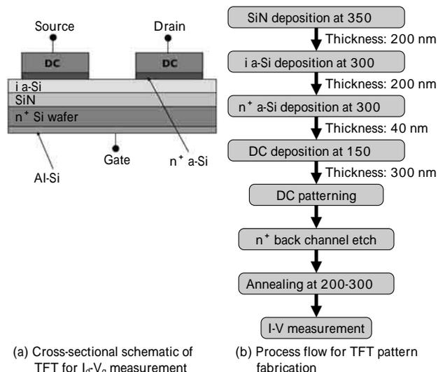
(a) Cross-sectional schematic of TFT for  $I_d$ - $V_g$  measurement (b) Process flow for TFT pattern fabrication
