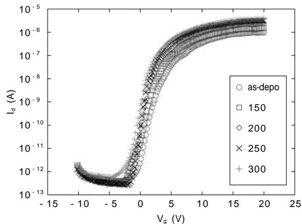
Fig.12 TFT  $I_d$ - $V_g$  characteristics after 150-300 °C annealing using Al-2at%Ni-0.35at%La and nitridation process
