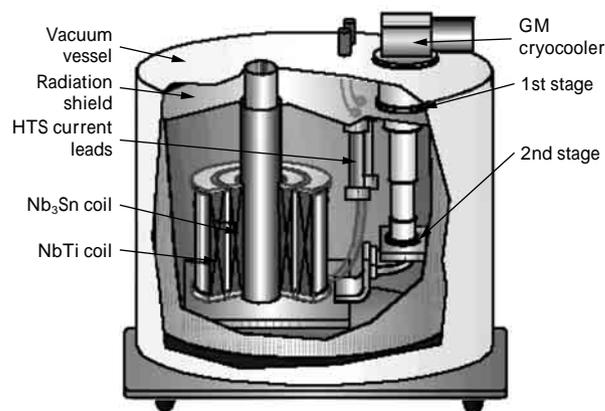
Fig. 1 Schematic view of cryogen-free superconducting magnet
