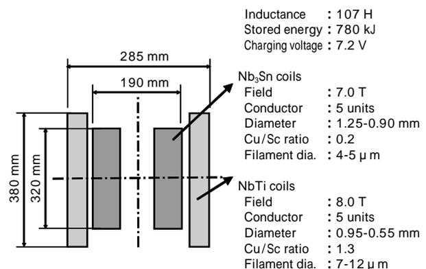
Fig. 3 Coil layout and wire specifications of 15T52mm cryogen-free superconducting magnet
