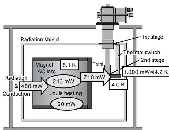
Fig. 4 Heat balance of 15T/52mm cryogen-free superconducting magnet
