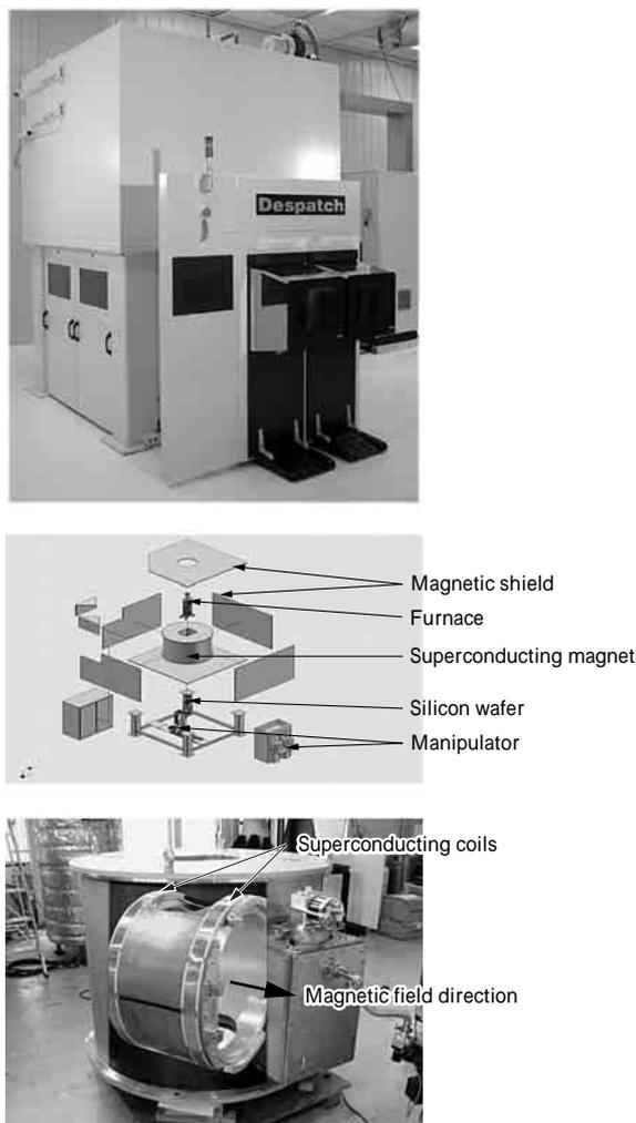
Fig. 6 Outside and inside view of annealing equipment for MRAM and superconducting magnet cut model
