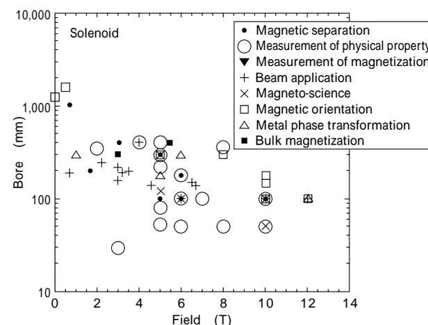
Fig. 5 Magnetic field/bore size and purpose of cryogen-free superconducting magnet
