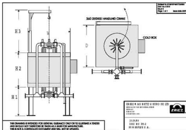
Fig. 7 Outside view of magnetic separation equipment for kaolin
