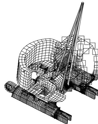
Fig. 2 Finite element model of hydraulic excavator
