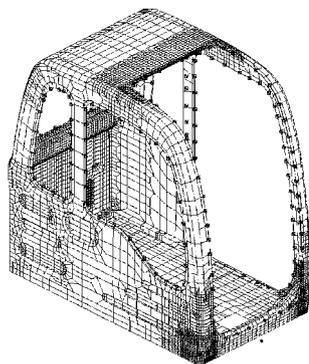
Fig. 6 Finite element model of cabin
