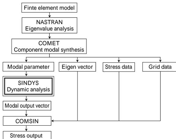
Fig. 1 System flow of dynamic strength analysis
