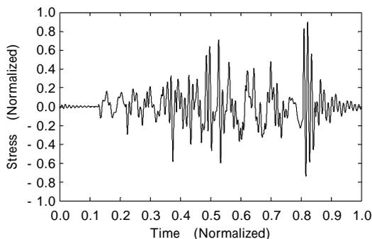
Fig. 4 Stress response of rough road simulation
