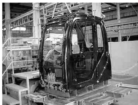
Photo 2 Oscillation test of cabin
