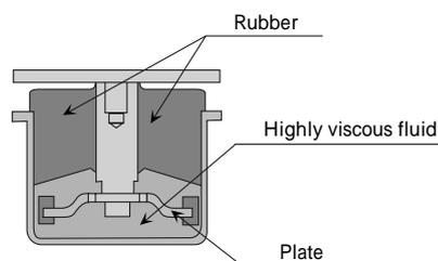
Fig. 5 Configuration of highly viscous fluid mount
