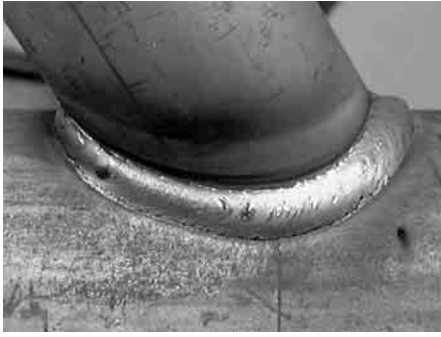
Photo 1 Appearance of welding bead
