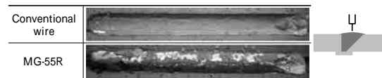
Photo 2 Comparison of slag detachability (Flat position welding, Plate thickness 16mm, Cooled to room temperature)
