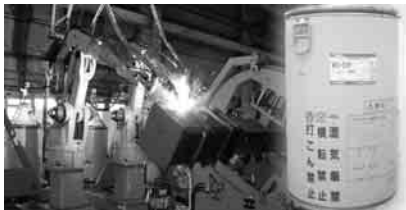
Photo 1 "ARCMAN" robot welding system and "MG-55R" wire
