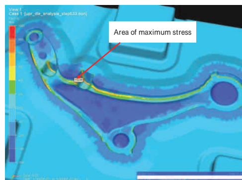
Fig.10 Stress distribution of forging dies obtained by FEM analysis
