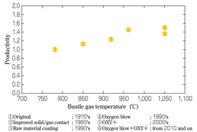
Fig. 6 Changes in productivity of MIDREX shaft furnace
