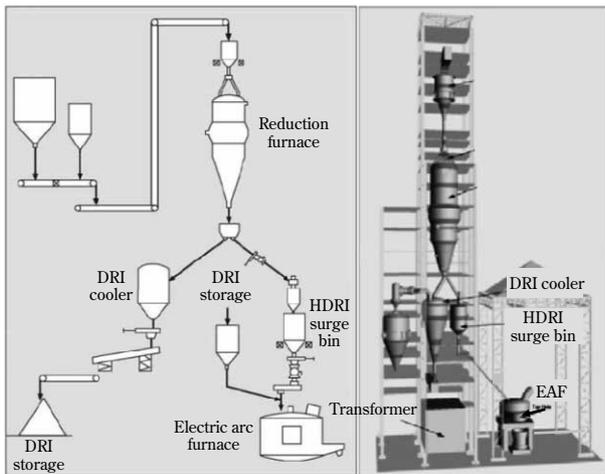
Fig.15 Material flow of HOTLINK and equipment arrange
