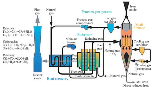
Fig. 3 MIDREX process flow sheet
