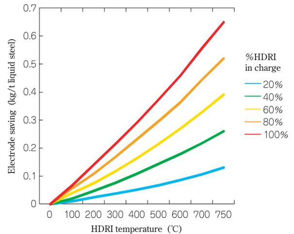
Fig.17 Correlation between HDRI temperature and electrode savings at EAF
