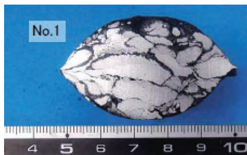
Fig. 6 Sectional view of HBI
