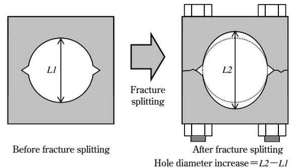
Fig. 3 Measuring method of hole diameter increase
