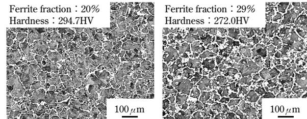
Fig. 6 Microstructures and hardness of Steel A and B
