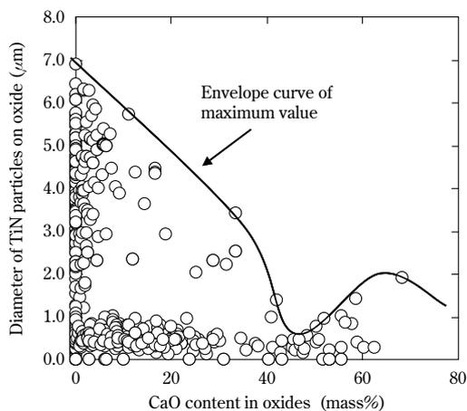
Fig. 2 Effect of CaO content in oxides on diameter of TiN particles
