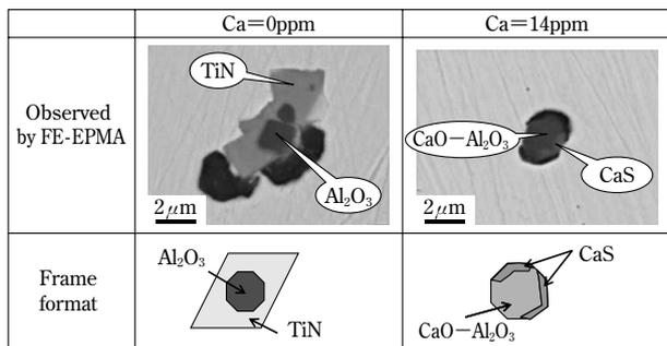
Fig. 1 Effect of Ca on inclusion morphology<sup>5)</sup>
