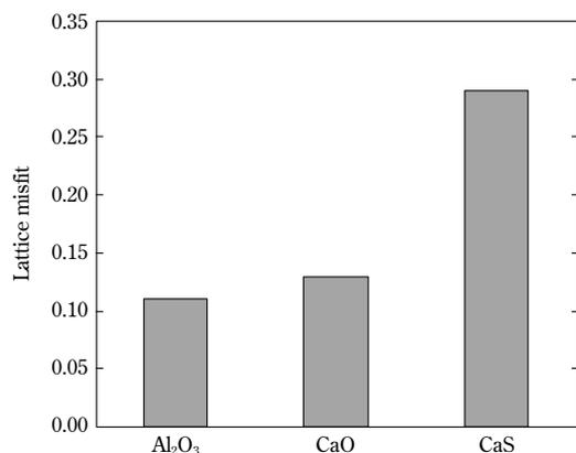
Fig. 5 Lattice misfit between TiN and inclusions
