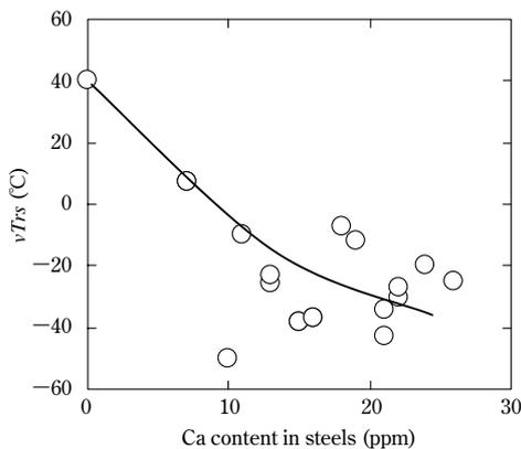
Fig. 7 Effect of Ca content on HAZ toughness
