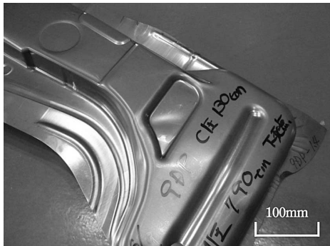
Fig.12 Example of wrinkle in test part (BHF=1,300kN 980DP steel)
