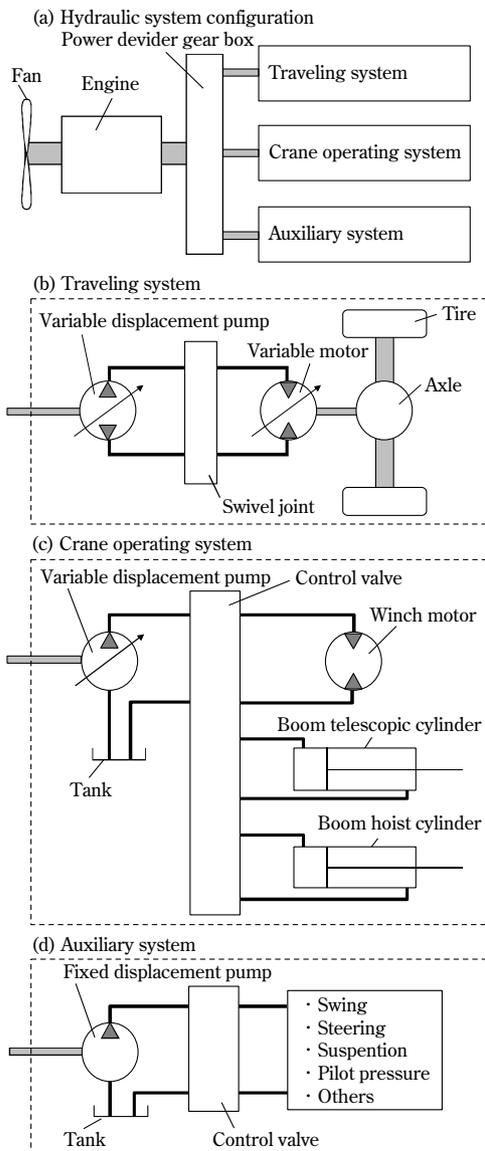
Fig. 1 Hydraulic system configuration of wheel crane
