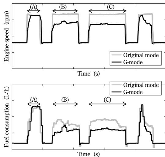
Fig.14 Engine speed and fuel consumption in G-mode
