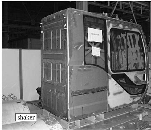
Fig.12 Shaker testing of cabin
