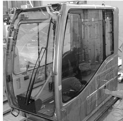
Fig. 9 Impact hammer testing of cabin
