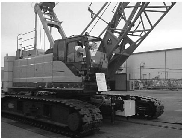
Fig. 1 Latticed boom crawler crane
