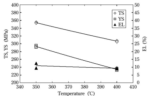
**Fig.10** Effect of forging temperature on mechanical properties
