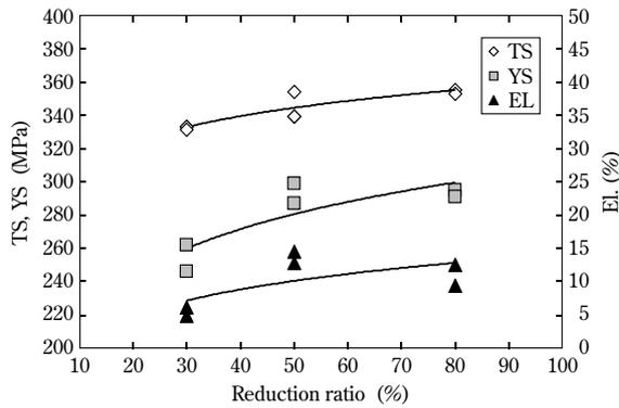
Fig.12 Effect of reduction ratio on mechanical properties
