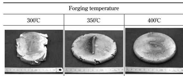
**Fig. 9** Effect of forging temperature on formability
