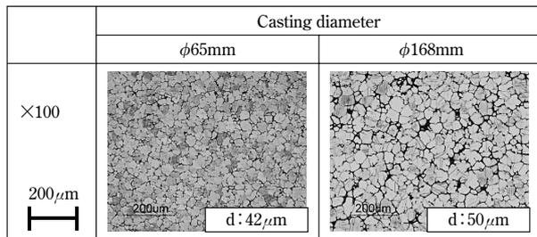
**Fig.15** Microstructure for each continuous casting diameter (as-cast)
