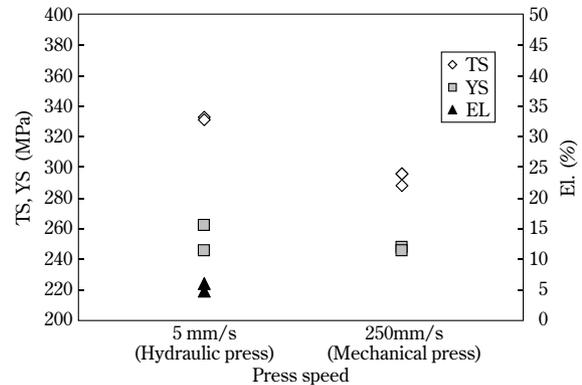
**Fig. 8** Effect of press speed on mechanical property
