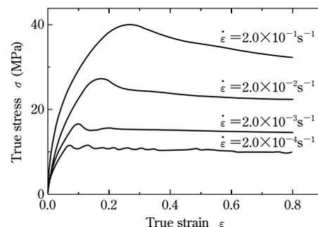
Fig. 3 Flow curves of Cu-P alloy billet samples compressed at  $1,073\text{K}$  at various true strain rates
