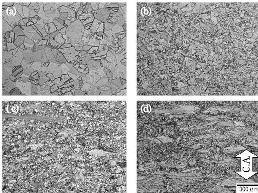
Fig.11 Microstructures in specimens deformed to  $\epsilon = 1.0$  at a strain rate of  $\dot{\epsilon} = 2.0 \times 10^{-1} \text{s}^{-1}$  at 1,073K; (a) 4NCu, (b) Cu-0.31Sn-0.024P, (c) Cu-0.66Sn-0.025P, (d) Cu-1.02Sn-0.025P
