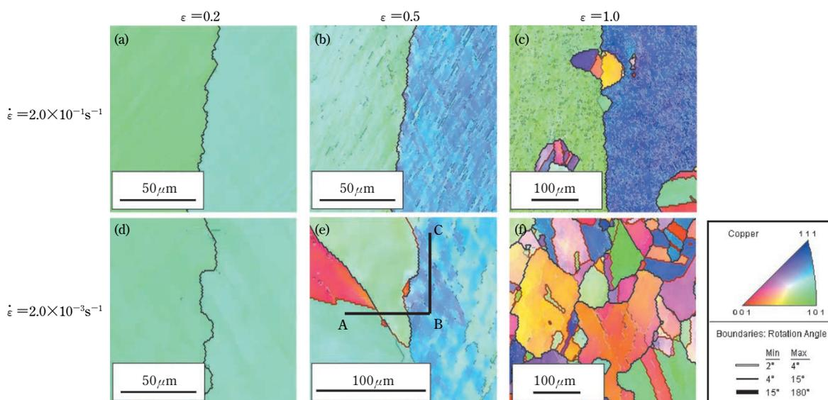
Fig. 8 OIM maps of microstructures in Cu-0.65Sn-P alloy bicrystals having  $[011]$  twist  $18^\circ$  grain boundaries deformed to various strains at 1,073K at strain rates of  $\dot{\epsilon} = 2.0 \times 10^{-1} \text{s}^{-1}$  and  $\dot{\epsilon} = 2.0 \times 10^{-3} \text{s}^{-1}$ <sup>13)</sup>
