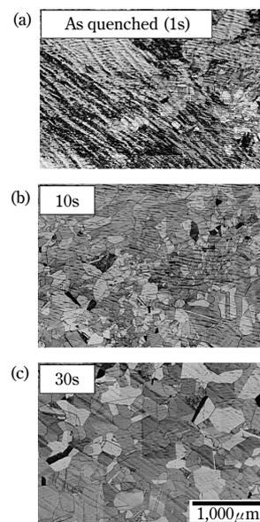
Fig. 6 Microstructure of Cu-0.65Sn-P alloy billet samples deformed to  $\epsilon = 0.8$  at 1,153K at strain rate of  $\dot{\epsilon} = 2.0 \times 10^{-1} \text{s}^{-1}$  (a), followed by annealing at 1,153K for 10s (b) and 30s (c)
