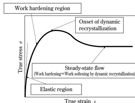
**Fig. 1** Typical flow curve in dynamic recrystallization
