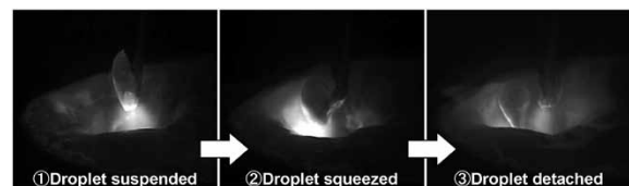
Fig.17 Droplet transfer of REGARC
