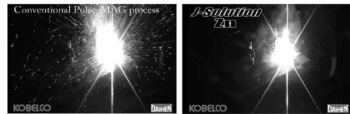
Fig.22 Use of J-Solution Zn for reduction of spatter generation
