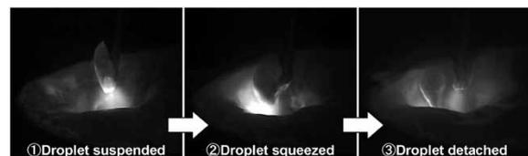
Fig.17 Droplet transfer of REGARC
