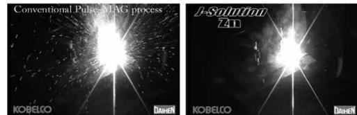
Fig.22 Use of J-Solution Zn for reduction of spatter generation
