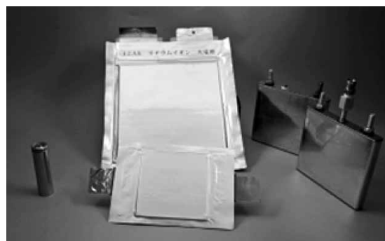
Fig. 1 Prototype cells for testing (cylindrical cell, laminate cell and prismatic cell from the left)
