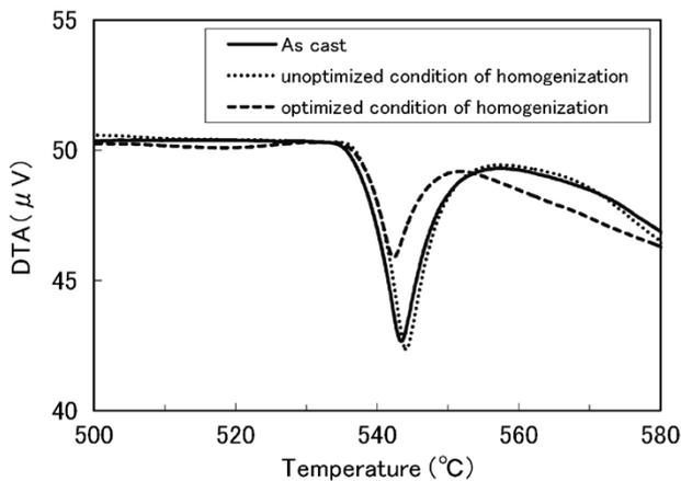
Fig. 5 Differential thermal analysis in each material condition
