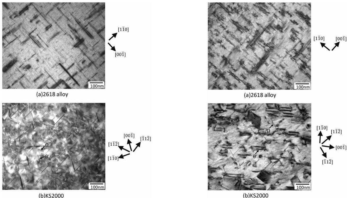
Fig. 1 Transmission electron micrographs after T61 artificial aging
