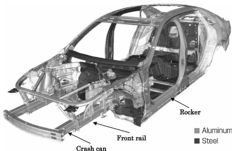
Fig.11 7000-series alloy extrusion applied to frames of production vehicles<sup>10)</sup>
