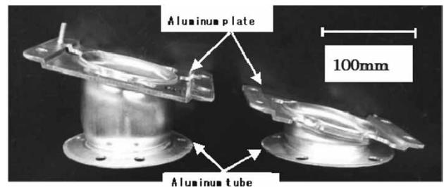
Fig. 8 Bumper stays produced by electro-magnetic forming
