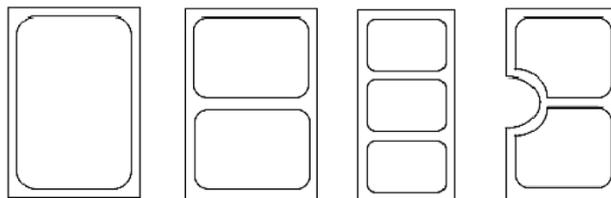
Fig. 4 Typical section type of bumper beam
