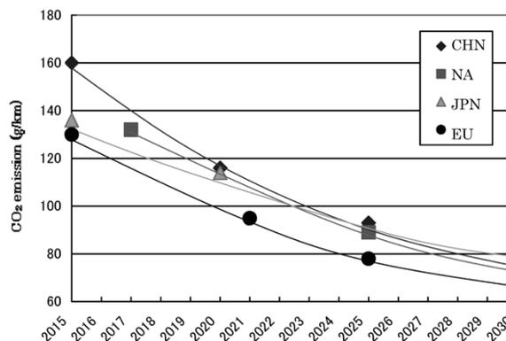
**Fig. 1** Transitions of standards being strengthened for fuel economy and CO<sub>2</sub> emission (fuel economy converted into CO<sub>2</sub> emission)<sup>3)</sup>
