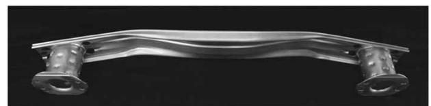
Fig. 9 Bumper system combining stay with beam
