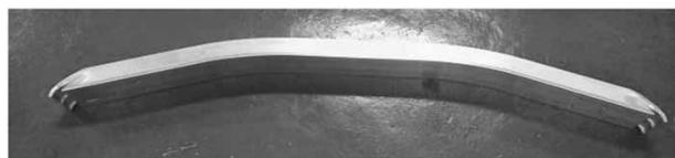
Fig. 6 Both-ends-formed bumper beam
