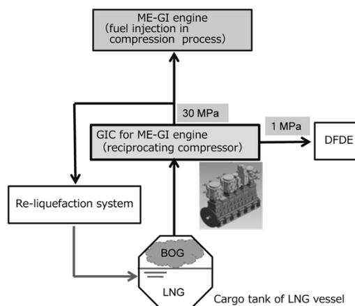
Fig. 1 Gas supply unit of ME-GI engine for LNG carrier
