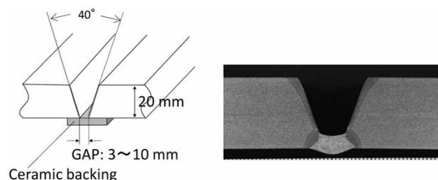
**Fig. 1** MAG penetration welding with ceramic backing material
