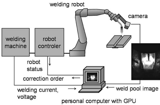
Fig. 2 System Configuration
