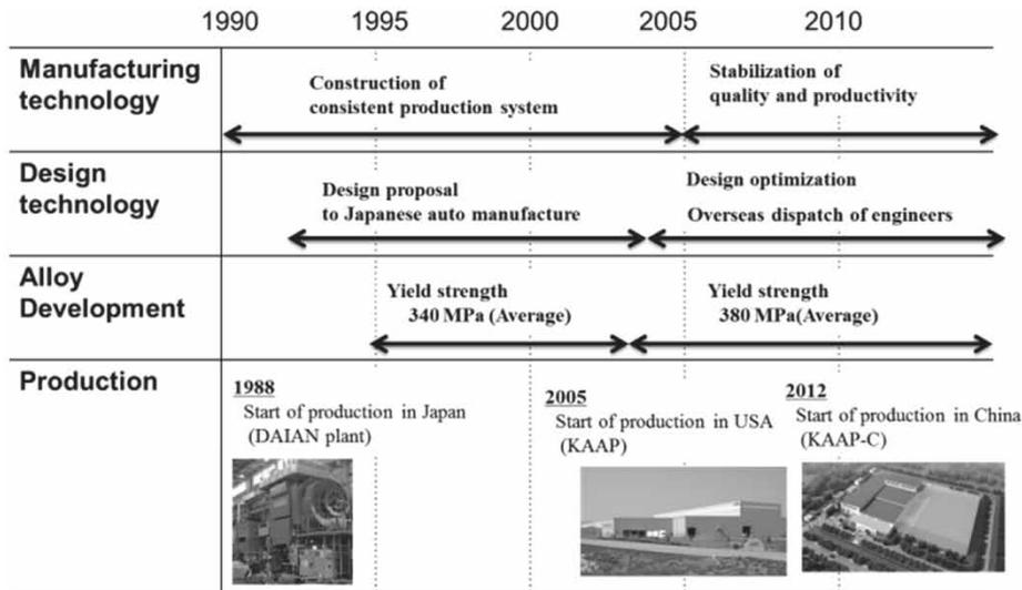
Fig. 6 History of technology development and global expansion of forged suspension of aluminum alloy in Kobe Steel<sup>10)</sup>
