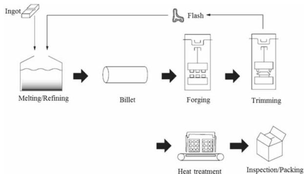
Fig. 5 Integrated production system for forged suspension of aluminum alloy in Kobe Steel<sup>9)</sup>
