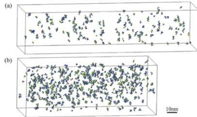
Fig.1 Mg and Si atoms found to be aggregated in an Al-Mg-Si alloy after (a) 10.8ks, (b) 360ks natural aging
