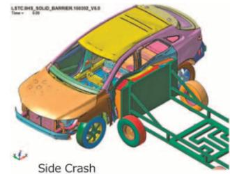
Fig.2 Simulation result of deformation of vehicle under side impact
