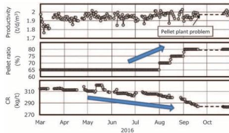
Fig.3 Transition of low coke rate operation
