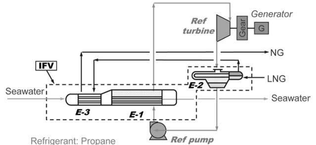
Fig. 5 Schematic diagram of process flow for LNG cryogenic power generation system (Rankine cycle)
