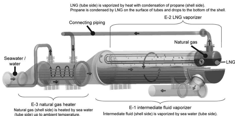
Fig. 3 Schematic diagram of intermediate fluid vaporizer (IFV)
