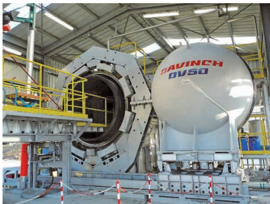
Fig. 5 Detonation chamber delivered to Poelkapelle, Belgium
