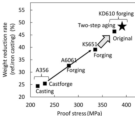
Fig.11 Relationship between proof strength and weight reduction rate of aluminum alloy<sup>8)</sup>
