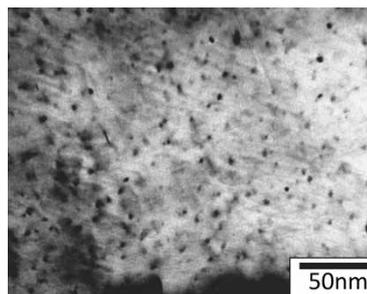
Fig. 9 TEM micrograph of specimen pre-aged at 160°C × 5 h and quenched at temperature of DSC peak 1 (Number density of precipitates:  $5.2 \times 10^{22}/m^3$ , size of precipitates: 6.7 nm)
