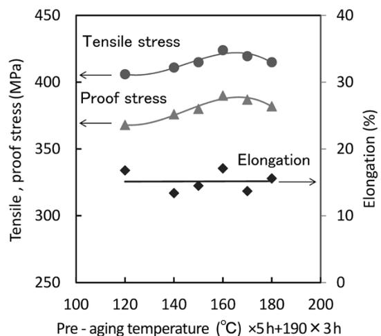
Fig. 4 Effect on tensile properties of pre-aging temperature
