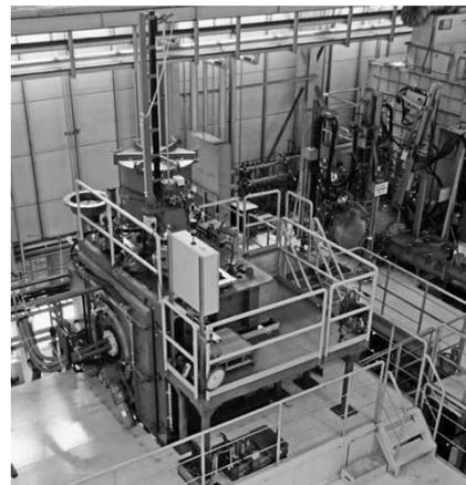
Fig. 7 Appearance of pilot-scale CCIM furnace
