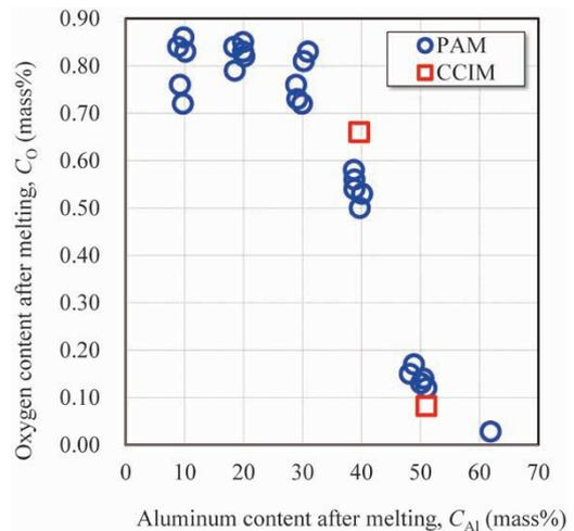
Fig. 3 Effect of aluminum content on deoxidation behavior in molten TiAl alloy
