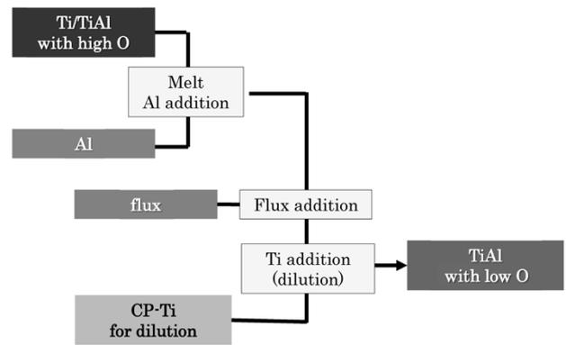
Fig. 6 Schematic diagram for TiAl alloy deoxidation process
