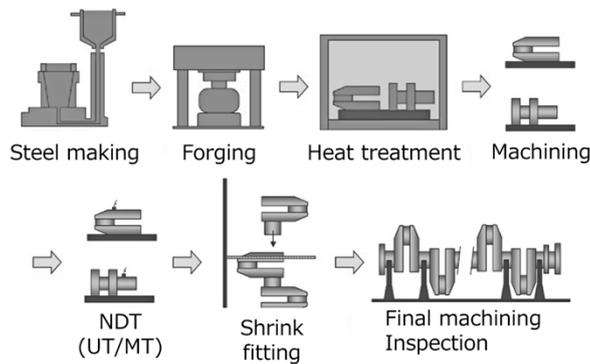
Fig. 1 Manufacturing process of semi-built-up type crankshaft
