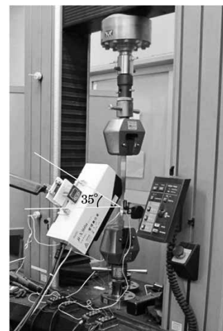
Fig. 2 Tensile test to confirm accuracy of X-ray stress measurement
