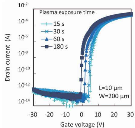
Fig. 3 Dependence of hydrogen plasma exposure time of Id-V<sub>g</sub> curve of top-gate TFT
