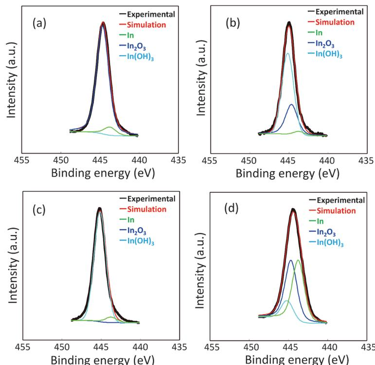
Fig. 5 In 3d<sub>5/2</sub> peaks of XPS spectra on the a-IGZTO thin film surfaces, (a) no plasma exposure, (b) after RIE, (c) RIE and argon plasma, and (d) RIE and hydrogen plasma exposure
