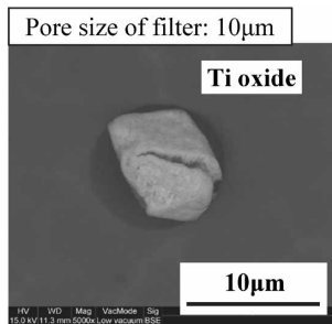
Fig. 5 Ti oxide on filter after mixed acid treatment
