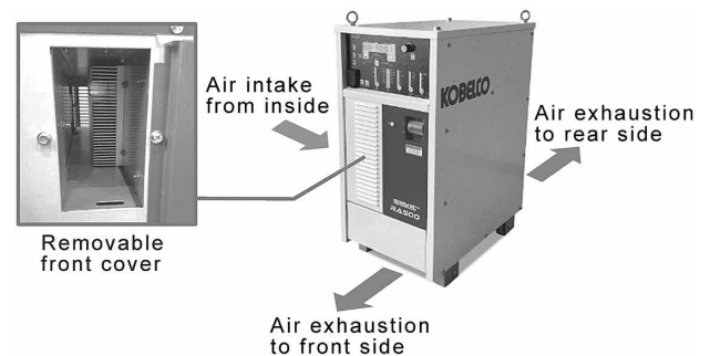
Fig. 3 Side flow structure
