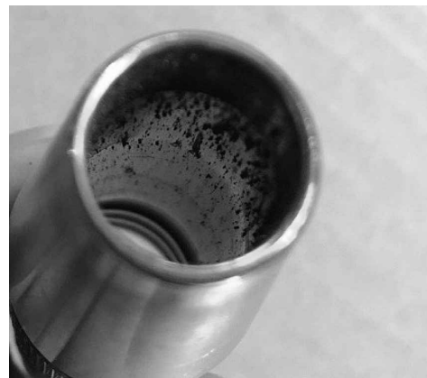
Fig. 3 Nozzle appearance after 40 minutes continuous of welding
