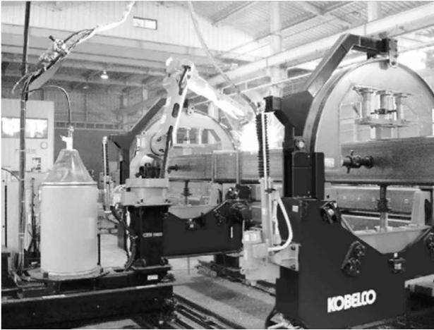
Fig.1 Structural steel large assembly welding robot system
