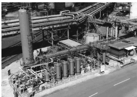
Fig. 2 Commercial CO-PSA plant installed at Kobe Steel's Kakogawa Works
