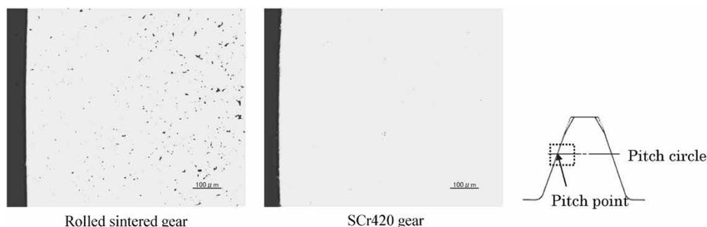
Fig. 2 Porosities and inclusions near pitch point
