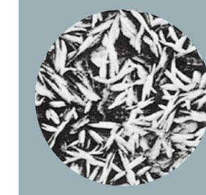
The phosphate film generated on the sheet surface assures outstanding paint adhesion, with an extremely smooth and attractive paint finish that only electrogalvanizing can provide.
