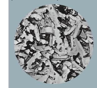
The alloying treatment diffuses iron particles in the coated surface to produce fine irregularities that ensure excellent paint adhesion.
