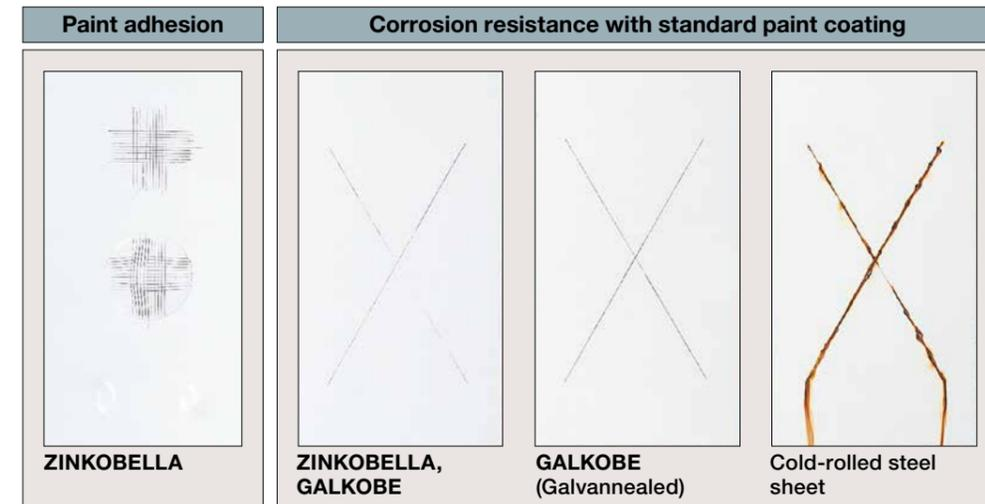
To reduce costs and environmental hazards, Kobe Steel also supplies galvanized steel sheet that has been chemical treated at the factory so that there is no need to prime the material before painting. In general, ZINKOBELLA (GX-GP treatment) and GALCOBE (Galvannealed) are most suitable for painting applications. For best results, choose a paint that is compatible with the chemical treatment applied.
