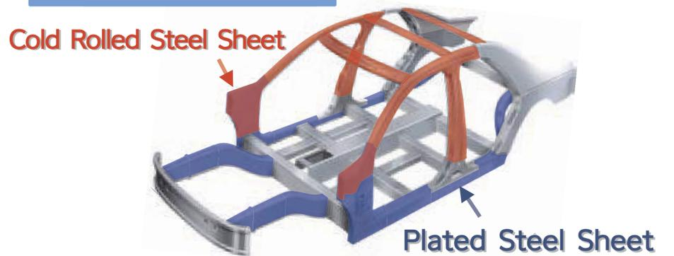
Contributes to the expansion in application of High Strength Steel to Body in white parts
