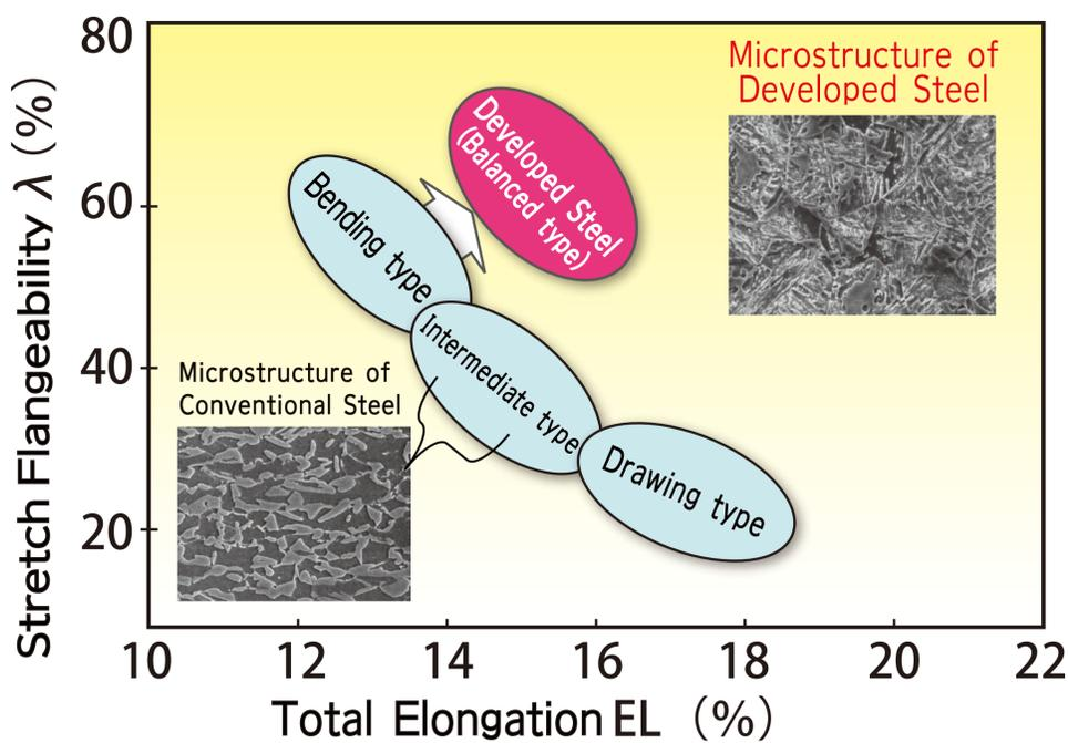
EL- $\lambda$  balance of the 980 N/mm<sup>2</sup>-grade High Tensile Strength Steel Sheet
