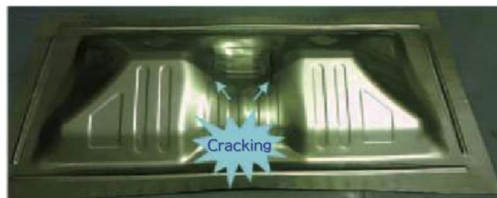
Example of Forming Simulating a Dash Panel
