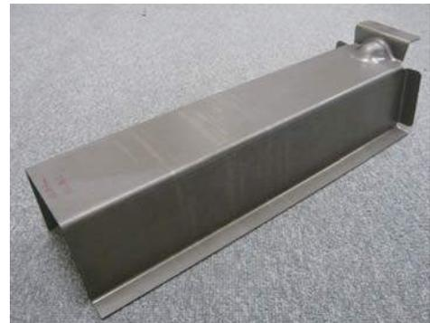
Prototype made of Ultra High-Tensile Strength 980 N/mm<sup>2</sup>-grade Steel
