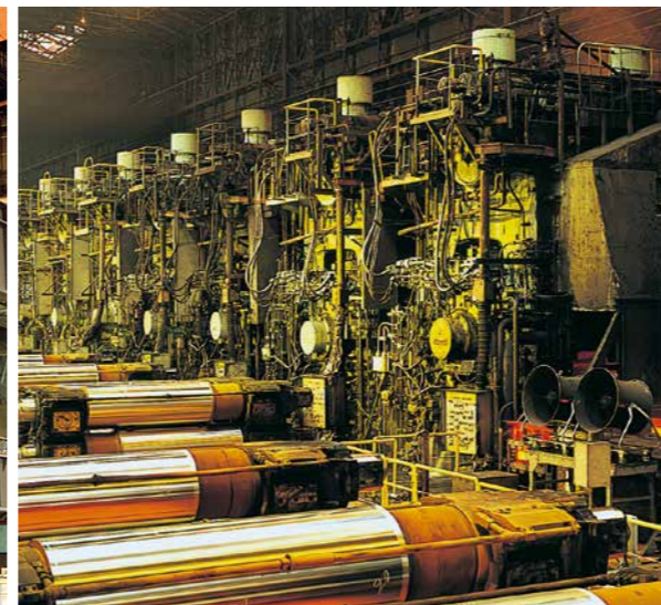
Hot strip mill
