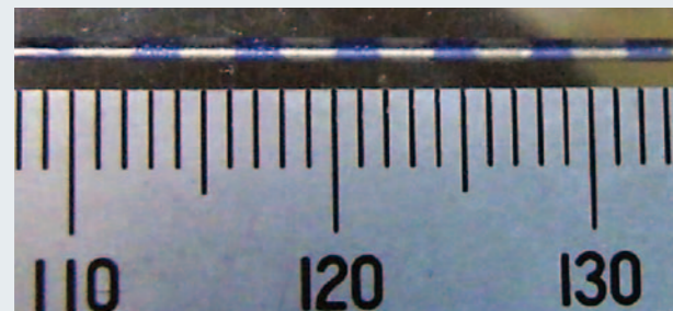
Example of liquid-liquid slug flow (single channel)
