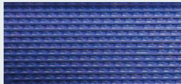
Example of gas-liquid slug flow (15 channels)
