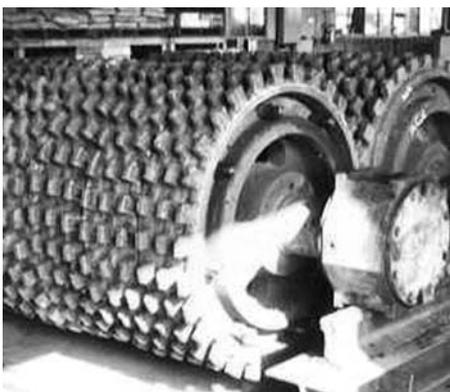
Figure 11: A typical application for **DWH-30** flux-cored wire and **HF-30** covered electrode of the high-Cr iron type: a double-roll crusher of mild steel.
