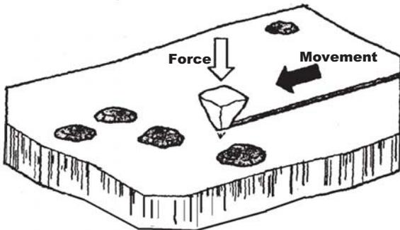
Figure 3: Scratching abrasion: The scratching action of granular solids against a metal surface under low or medium stresses causes gradual flaking of the metal. (Source: Welding Design & Fabrication)
