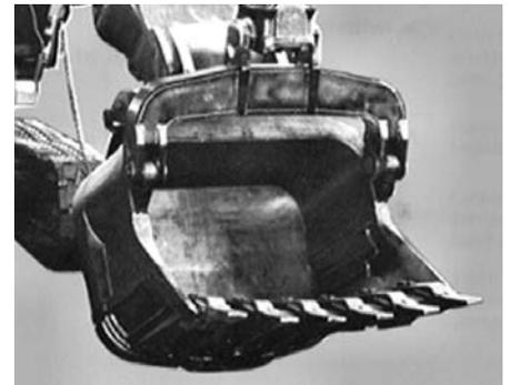
Figure 12: A typical application for **HF-950** covered electrode of the W-carbide type: dipper teeth of high-Mn steel.
