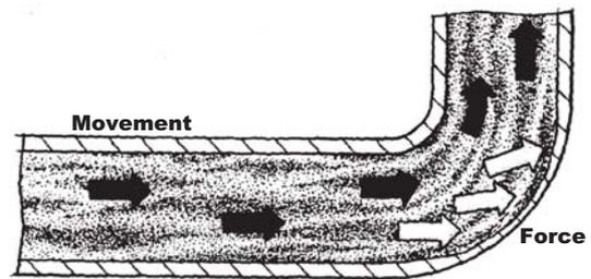
Figure 6: Erosion: Contact with fluids can cause removal of metal. Depending on the fluid the erosion can be classified as sand erosion, cavitation erosion, erosion corrosion, and rain erosion. (Source: Welding Design & Fabrication)
