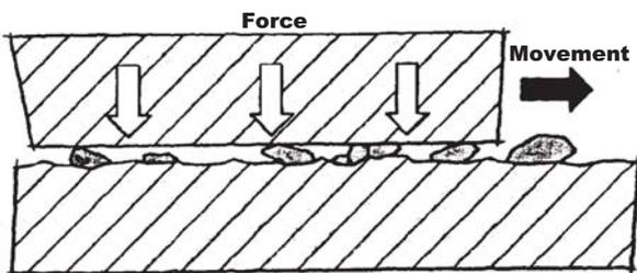
Figure 4: Grinding abrasion: The grinding action of granular solids indenting a metal surface under medium or high stresses causes gradual removal of the metal. (Source: Welding Design & Fabrication)
