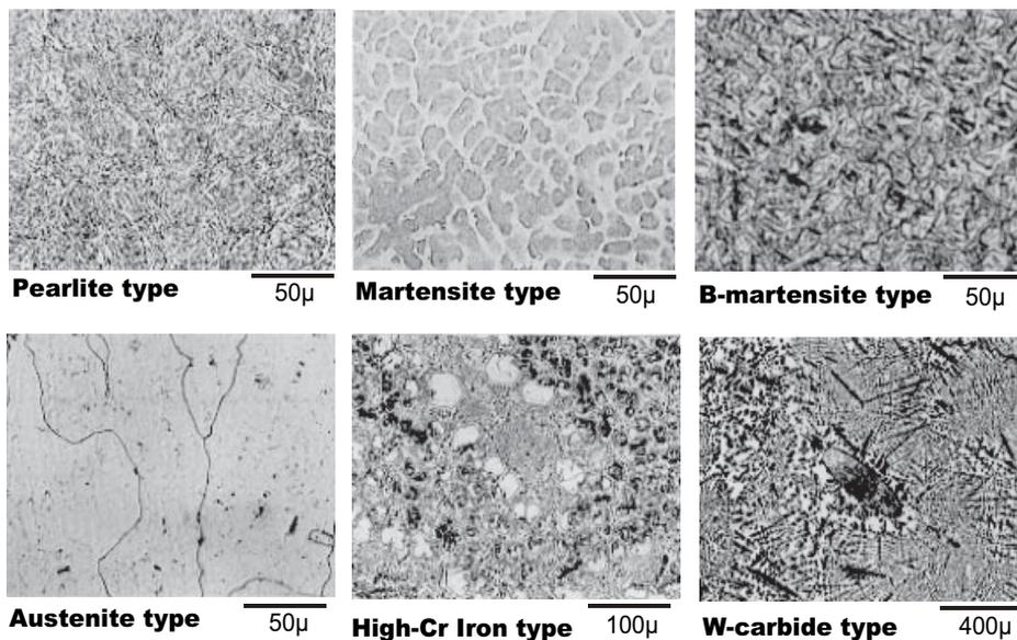
Figure 7: Typical microstructures of different hardfacing deposited metals [Refs. 1 and 2]
