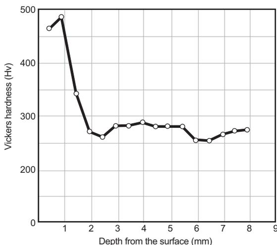
Figure 1: Hardness distribution of the 13%Mn cast steel mantle of a gyratory crusher after operation [Ref. 1].
