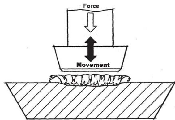
Figure 2: Impact wear: Repeated striking of metals causes fatigue and the removal of the lower-strength metal. (Source: Welding Design & Fabrication)
