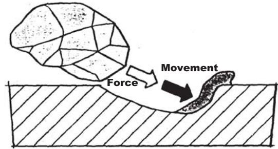
Figure 5: Gouging abrasion: A collision of rocky solids against a metal surface under high stresses causes quicker, larger-mass removal of the metal by shearing stresses. (Source: Welding Design & Fabrication)
