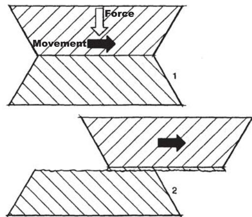
Figure 1: Adhesive wear: Adhesion in the metal interface causes detachment of a lower-strength metal. (Source: Welding Design & Fabrication)
