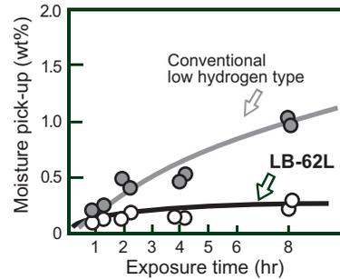
Figure 4: Test results of LB-62L and conventional low-hydrogen electrode on moisture pick-up under the controlled atmosphere: 30°C x 80%RH.
