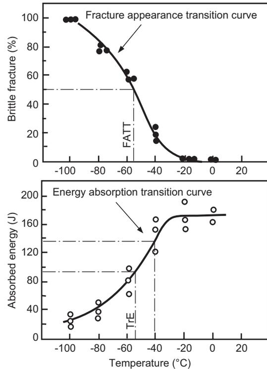
Figure 1: Energy absorption transition and fracture appearance transition curves of mild steel or low alloy steel welds.
