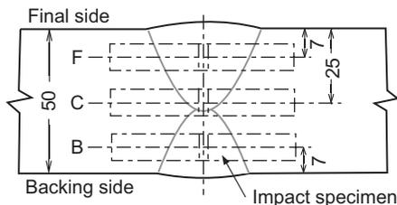
Figure 1: Charpy impact properties of LB-80L (4.0mm $\varnothing$ ) weld metal (Base metal: 50-mm-thick 780-MPa high tensile steel of K-TEN780 with double-V groove; Welding position: Vertical-up; Welding parameter: 120Amp./22V; Heat input: 2.0kJ/mm; Preheating and interpass temperature:  $150^{\circ}\text{C}$ ).
