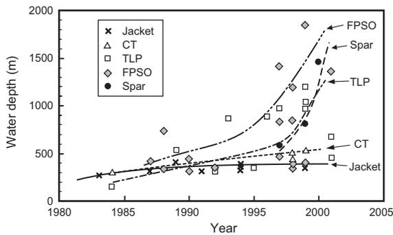
Figure 2: Water depth transition for offshore structures [Ref.1]
