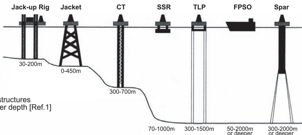
Figure 1: Varieties of offshore structures and their working water depth [Ref.1]
