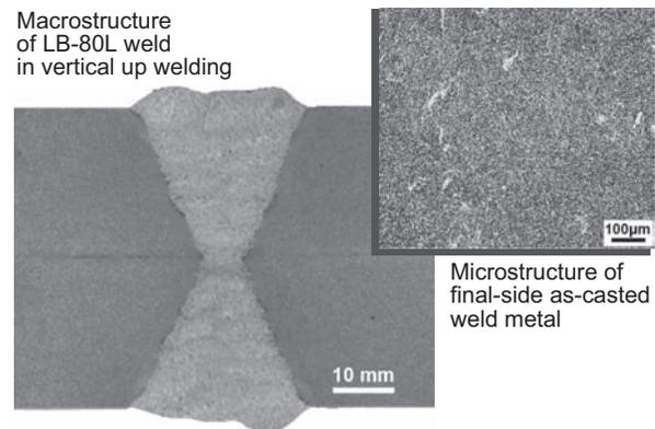
Figure 2: Typical macroscopic and microscopic structures of LB-80L weld (Refer to Figure 1 for welding conditions).
