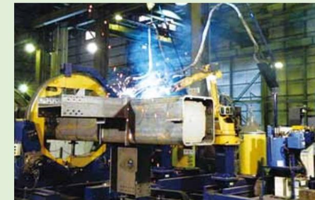
Figure 6: Application of robotic welding system for hull assembly in shipbuilding
