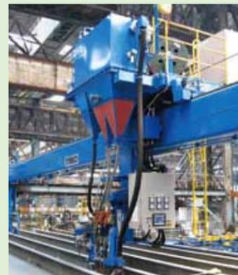
Figure 2: FCB™ equipment for one side welding
