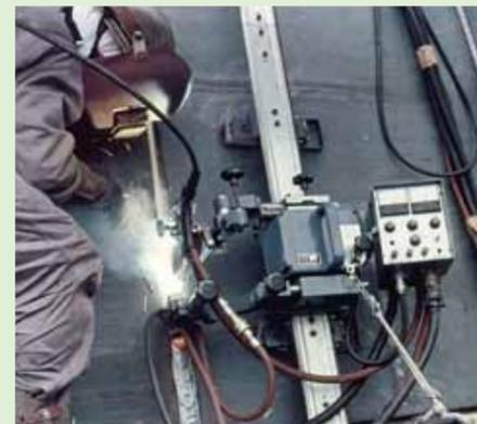
Figure 4: Welding site of TRIFARC™ process
